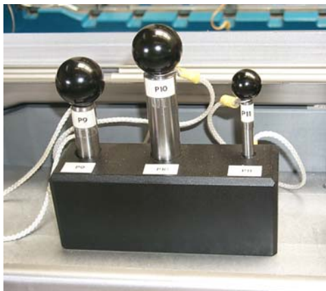
Fig. 6: Deposition for checking pins
